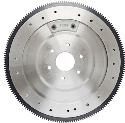
1646083 FOR 429-460BB EXTERNAL BALANCE 28 IN/OZ.W/6028S COUNTERWEIGHT
