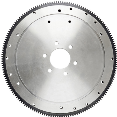
1645582 FOR OLDS 307, 350-455 1968-1985 & 100 1968-1970 ZERO/NEUTRAL/INTERNAL BALANCE
