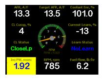
AIR/FUEL RATIO Multi-Gauge Engine below 160° F (NoLearn)
