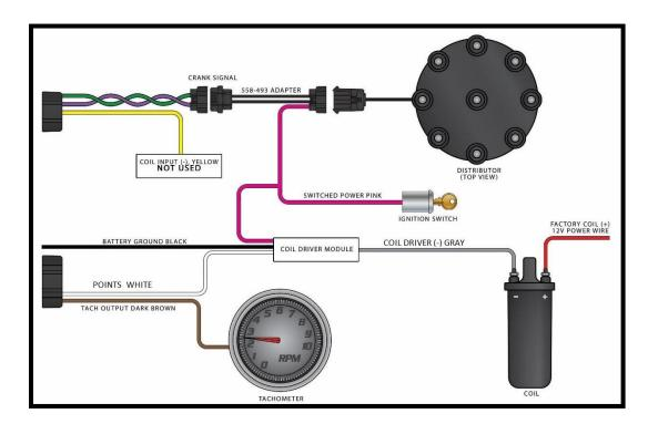
WIRING W/ Holley Dual Sync Distributor and CAPACATIVE DISCHARGE BOX (Such as MSD 6AL)
