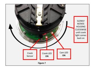
Turn the housing **clockwise** until the Crank LED comes back **ON** (**Figure 7**). Stop at this point. This will position the distributor close to where it needs to be. Install and snug the distributor clamp down at this point.
