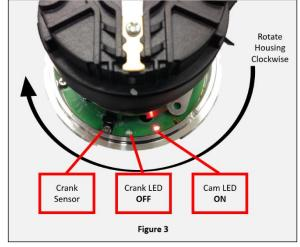
For engines that have the rotor rotating **clockwise**, turn the housing until the rotor contact is pointed at the black crank position sensor (**Figure 2**). Both the cam and crank LED should be illuminated (**ON**).
