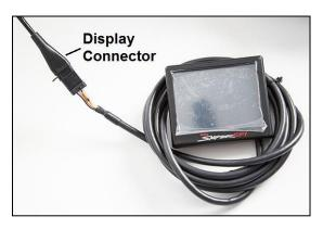
Note: If the 3.5" Touch Screen LCD Display needs to be unhooked from the Sniper EFI. Depress the lock tab on the male side of the connector as show in the following pictures.
