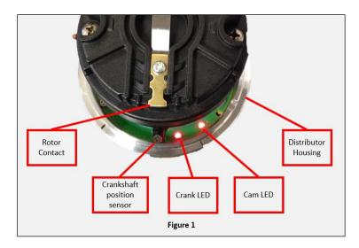
**NOTE:** All adjustments will be made by rotating the distributor housing only. **DO NOT ROTATE THE CRANKSHAFT** as it should remain at 50 degrees BTDC.
