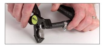
2. Install the fitting, by sliding the fitting into the hose. Make sure the hose seats flush with the fitting. (Figure 45-2)
