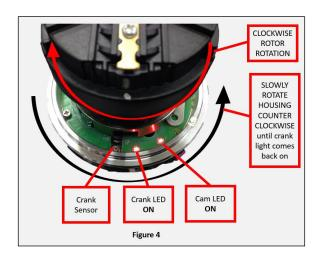
Then slowly turn the housing **counter-clockwise** until the Crank LED comes back **ON** (**Figure 4**). Stop at this point. This will position the distributor close to where it needs to be. Install and snug the distributor clamp down at this point.
