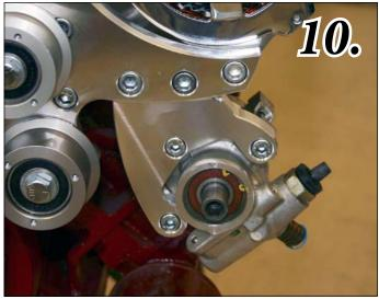
**Photo 11.** Slide the Alternator Fan (221-A) over the alternator shaft followed by the Alternator Pulley (208-A). Use the lockwasher (S685) and lock nut then tighten (We recommend a impact for installation of alt pulley, impact to 90 ft, pounds).
