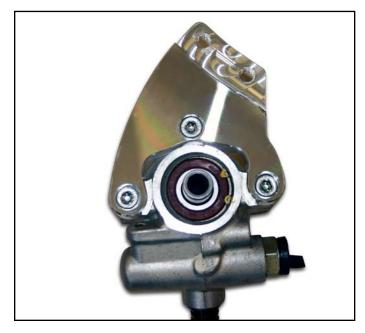
**Photo-12** Install the Power Steering Bracket to the Main front bracket Using two 3/8 x 1" SHCS (S248).
