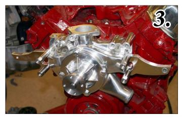
**Photo-4** Install The Main Face Plate (40721-A) using (4) (S244)  $\frac{3}{8}$  x  $\frac{3}{4}$  " SHCS thru the four counter sunk bolt holes in the front of the plate and into the four Stainless Threaded Spacers.
