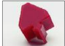
3.9103 G.M. style pull thru bump stop. Fits many 1978-88 G.M. RWD cars and trucks. 1 5/8" tall x 1 13/16" long x 1 15/16" wide. 2 per set.
