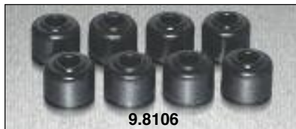
9.8106 I.D.— 3/8 " , Nipple O.D.— 5/8 " , O.D.— 1 " , O.A.L.— 11/16 " For cars & mini trucks. 8 per set.
