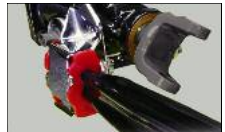
Performance Torque Arm Bushings connecting the differential to the transmission.
