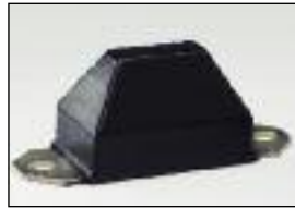
9.9137 2 bolt style, fits '76-86 Jeep CJ5/7 front & rear positions. 1 7/8" tall x 5" overall length x 1 3/4" wide. Accepts 3/8" dia. bolts with center to center of 4 1/4" max. to 4" min. 2 per set.
