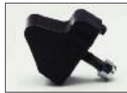
9.9150 G.M. style bump stop. Fits many 1970-99 G.M. cars & trucks. 2" tall x 2 1/4" long x 1 1/16" wide. 1" long stud with a 5/16" dia. locating pin at 1" offset. 2 per set.
