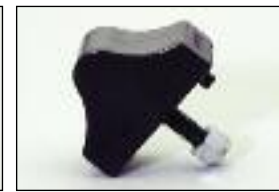
9.9154 Single hump early GM style. Lower control arm direct replacement for '64-72 Chevelle, '68-72 Nova and '67-69 Camaro. 1 1/8" wide x 2 1/2" long x 1 11/16" tall. 2 per set.
