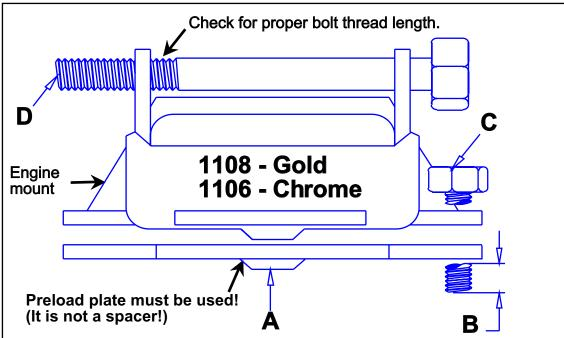
Note: ENERGY SUSPENSION does not supply bolts in set due to the many different applications.
